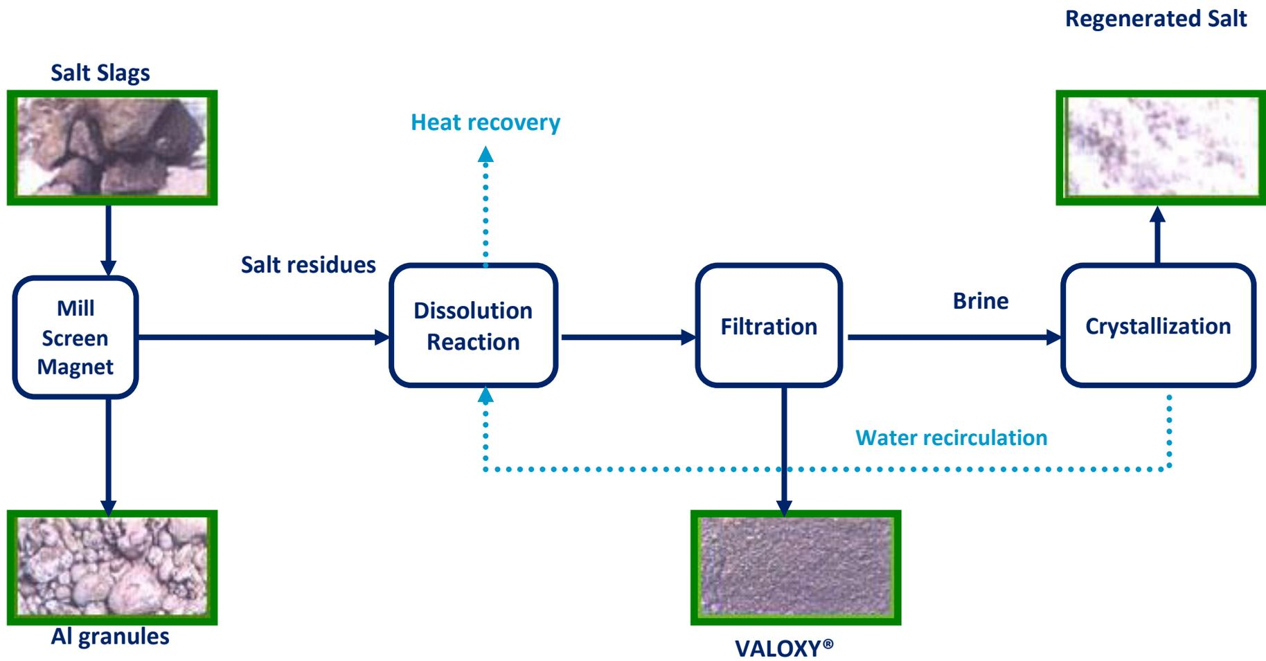
Figure 5. RVA process flow chart showing three main outputs: aluminium granules, salt and VALOXY
