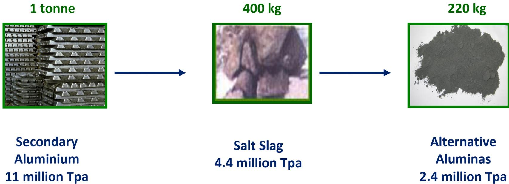
*Figure 4. Estimated global potential of alternative aluminas*
