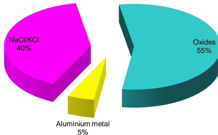
*Figure 3. Typical composition of salt slag*
