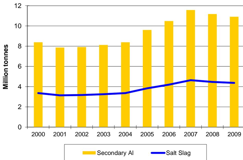
Figure 2. World arisings of salt slag - a function of secondary aluminium production
